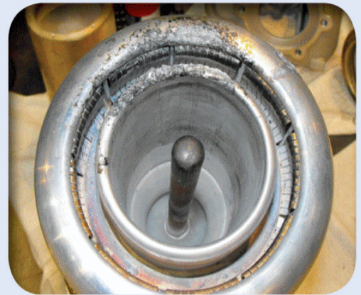
SF 6 Puffer Arcing and Main Contact
