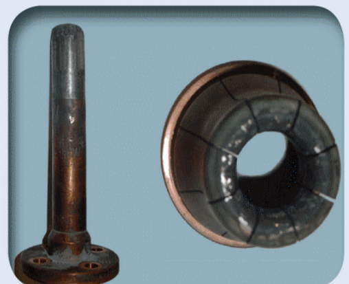
SF 6 Generator Circuit Breaker Arcing Contact
