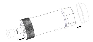
2. Install the transmitter to the mechanical coupling and tighten gently by hand. Then use a 30mm wrench to tighten the connection. Use a sufficient force to achieve a tight installation (recommended 10-15Nm). The system must be leak-free for accurate measurement.
