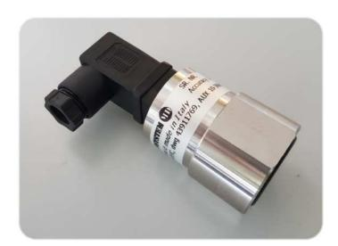
Type A transmitters are based on bridge resistance variation principle and the primary element is directly deposed on reaction mechanics by a silk screen-thick film process .
